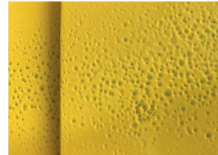
Wetting impairments due to insufficient adhesion of the powder
