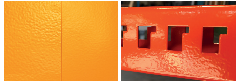
Excessive coating thickness can lead to orange peel skin
