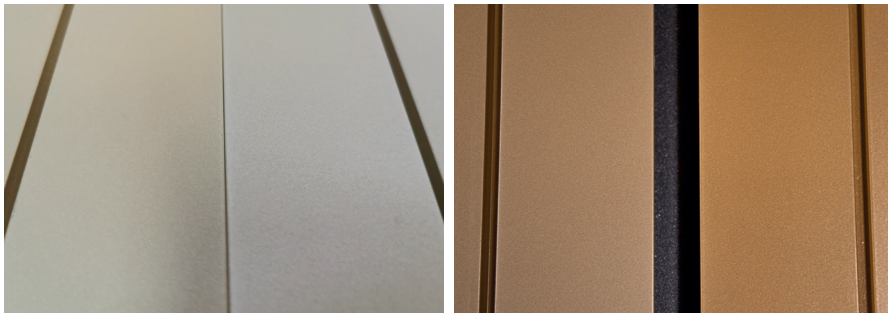
Color deviations from effect powder coatings
