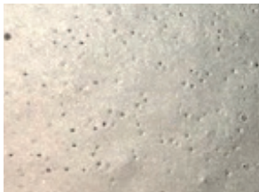
Needle sticks in coating surface
