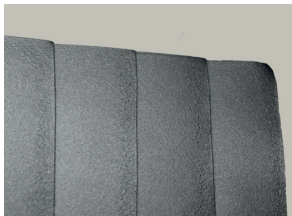
Picture frame effect at edges
