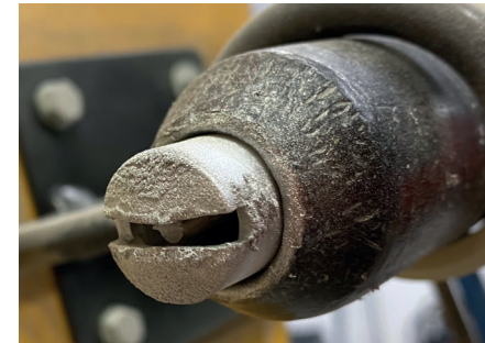
Deposits caused by sintering on the spraying nozzle
