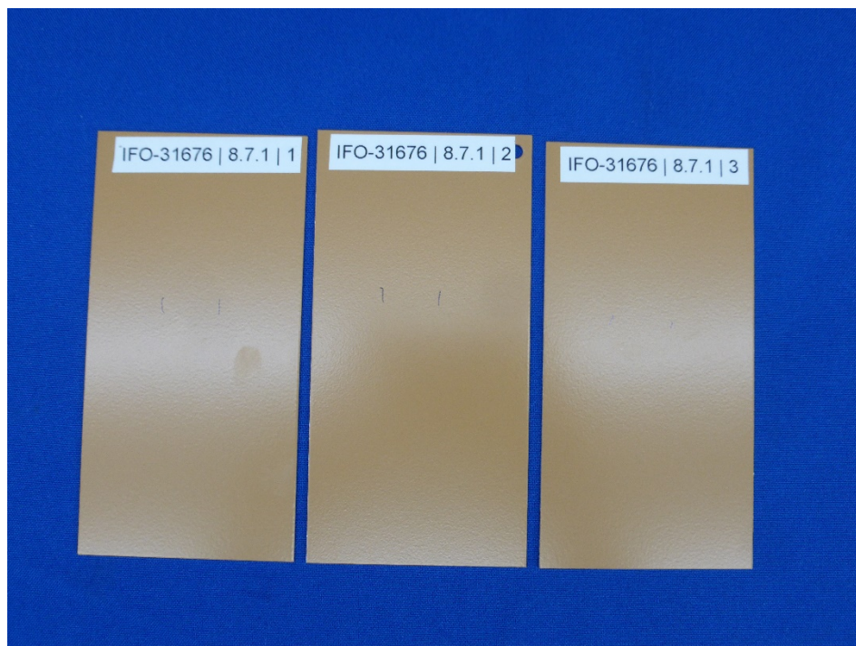
Figure 8 – Samples after Muriatic Acid Resistance test (see Ch. 2.7.1: Tests acc. to AAMA 2605-20, Ch. 8.7.1)
