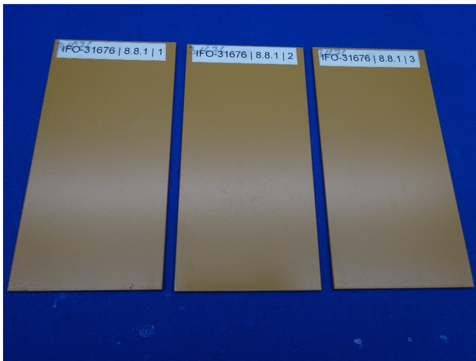
Figure 13 – Samples after Humidity Resistance test (see Ch. 2.8.1: Test acc. to AAMA 2605-20, Ch. 8.8.1)
